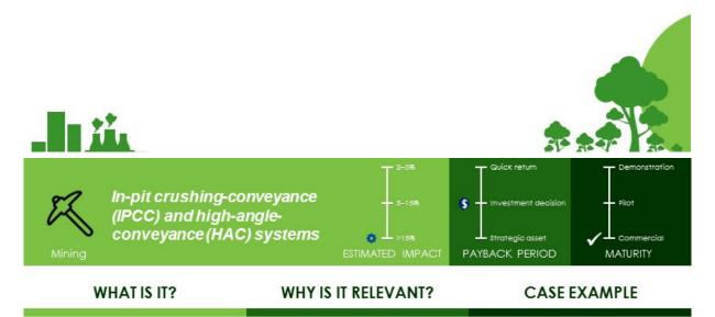
In-pit crushing involves processing ore using portable crushers. High-angleconveyance systems transport ore and waste products out of the mine. The main benefit is that instead of using large fleets of dump trucks–and all the fuel they consume and the emissions they produce–rock is crushed in the pit, and then conveyors carry it out.
